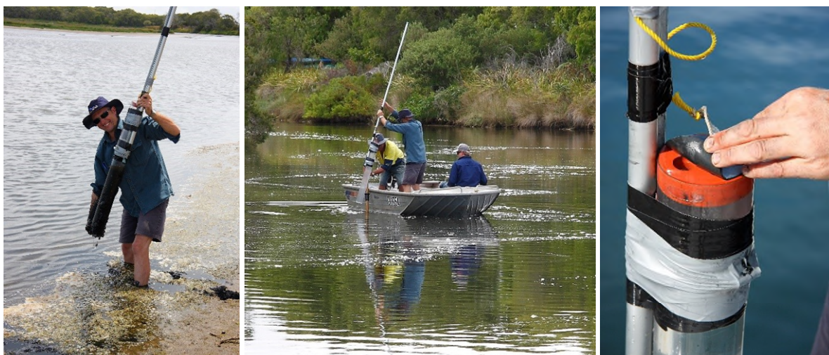
Figure 6.2 Sampling MBOs using a sediment coring device.
