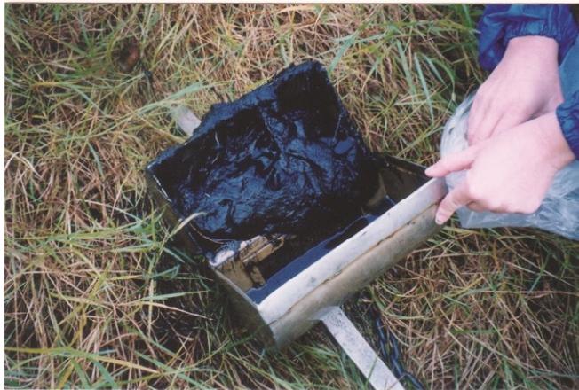
Figure 6.3 Sampling MBOs using a Van Veen grab sampler.
