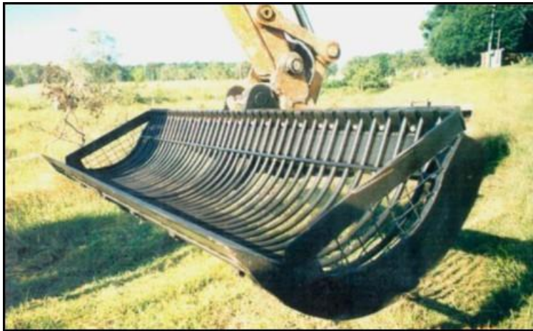
Figure 5.6 Example of a reed bucket used to remove MBOs from waterways.
