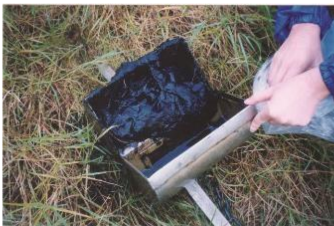
Figure 5.3 Sampling MBOs using a Van Veen grab sampler.
