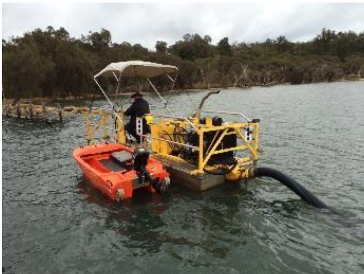
Figure 5.7 A small-cutter suction dredge removing MBOs from the Peel-Harvey Estuary, Western Australia.
