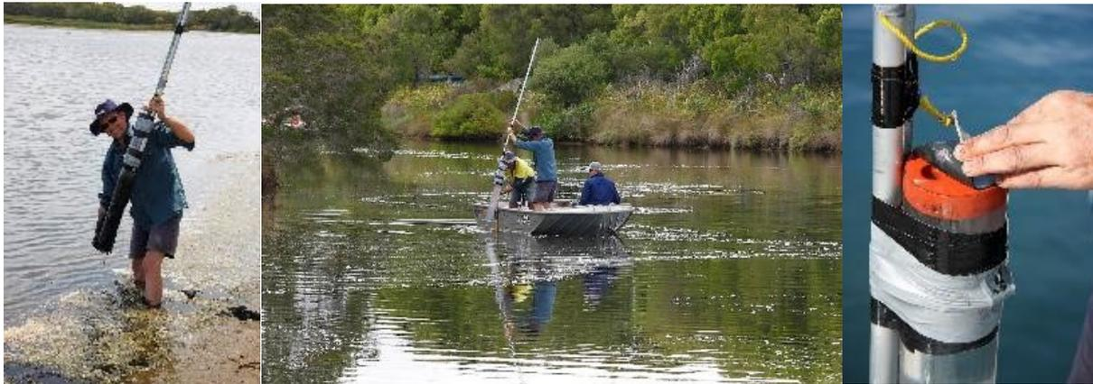
Note: Left and middle image of the coring device and right image of the water outlet at the top of the device.
