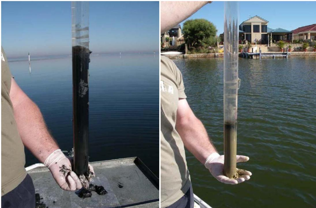
Note: The sediment profiles show variation in MBO thickness within waterways.
