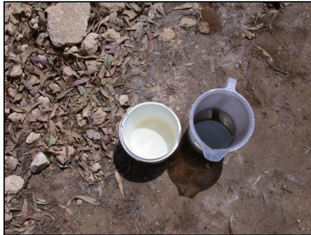
Figure A5 Dredge effluent pre and post dosing.
